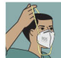
Remove by pulling the bottom strap over back of head, followed by the top strap, without touching the respirator.
