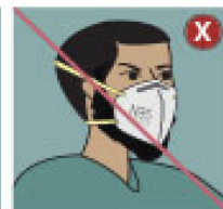
Do not allow facial hair, jewelry, glasses, clothing, or anything else to prevent proper placement or to come between your face and the respirator.
