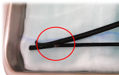
Tissue at tip :cleaning process inadequate
