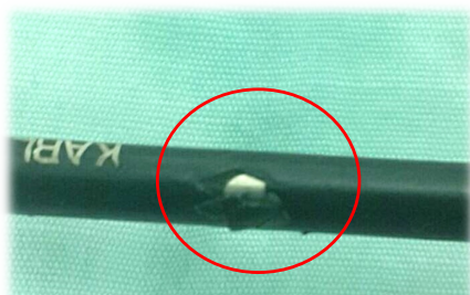
Instrument damage :inspection process inadequate
